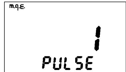
Pic.11 Regulation of number of pulses for every wheel turn
